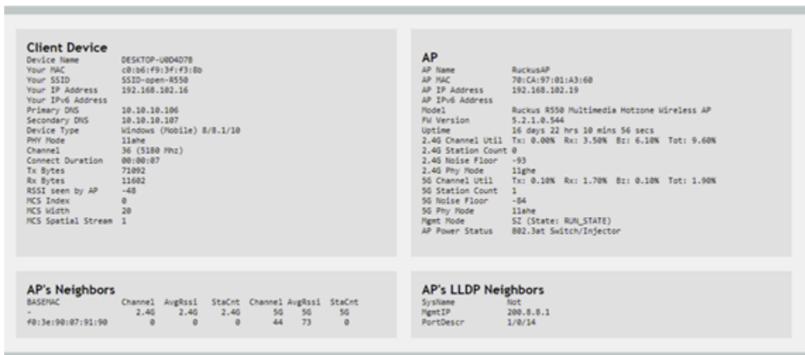
FIGURE 370 Viewing Diagnostic Information in WPA2 WLAN
