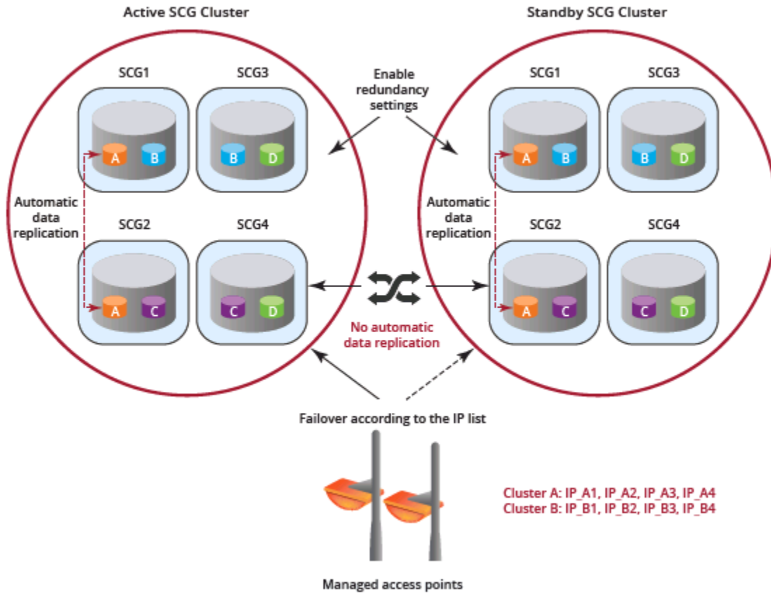
FIGURE 74 Cluster Redundancy for Active-Standby Mode
